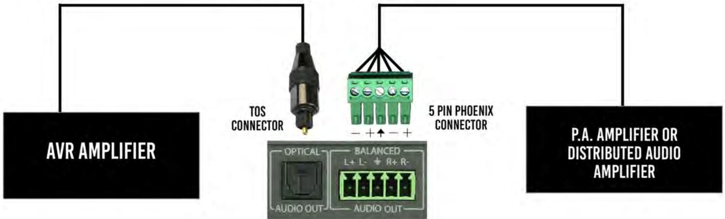
1. LINE IN - Balance Mono Analog Audio Input (use + and Ground  $\perp$  )
