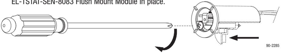
8. Reinstall the metal disk on the module.
