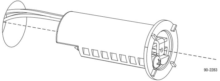
7. Tighten the screw as shown below to secure the EL-TSTAT-SEN-8083 Flush Mount Module in place.
